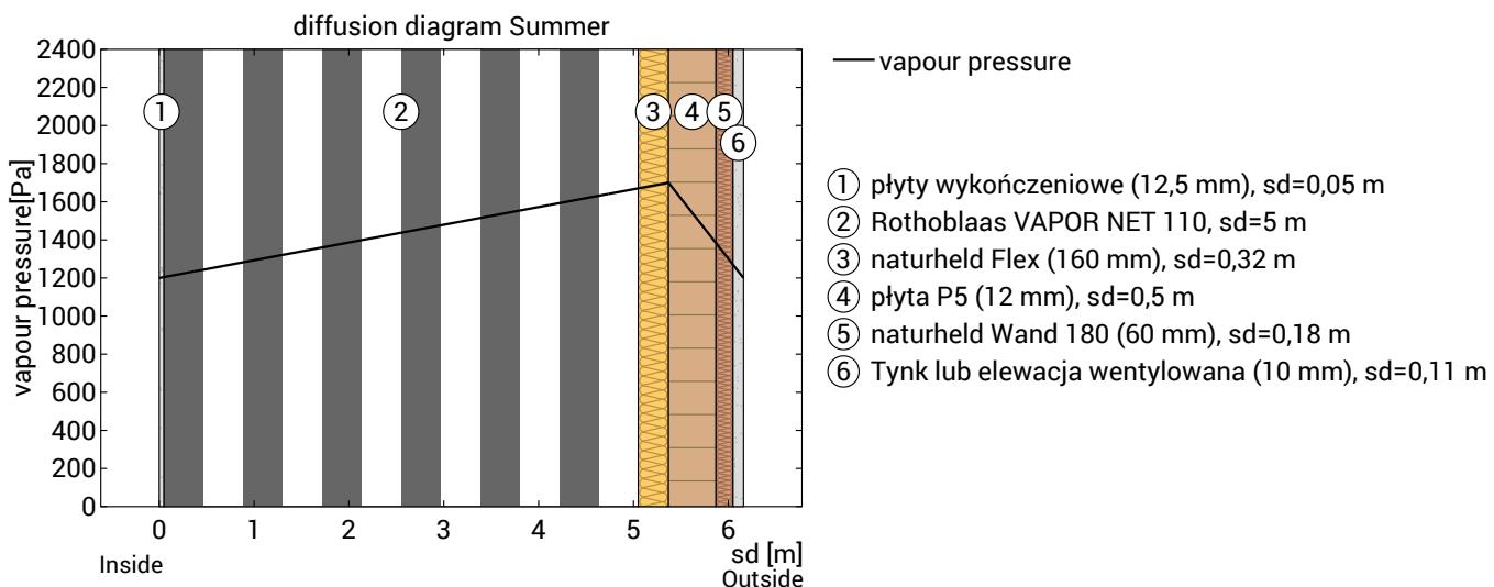
Condensate-free component: The maximum possible evaporation mass for the drying reserve is calculated. Consider the level that has the lowest evaporation potential in the dew period, at  $sd=5,37 \text{ m}$ ;  $x=17,28 \text{ cm}$ :
