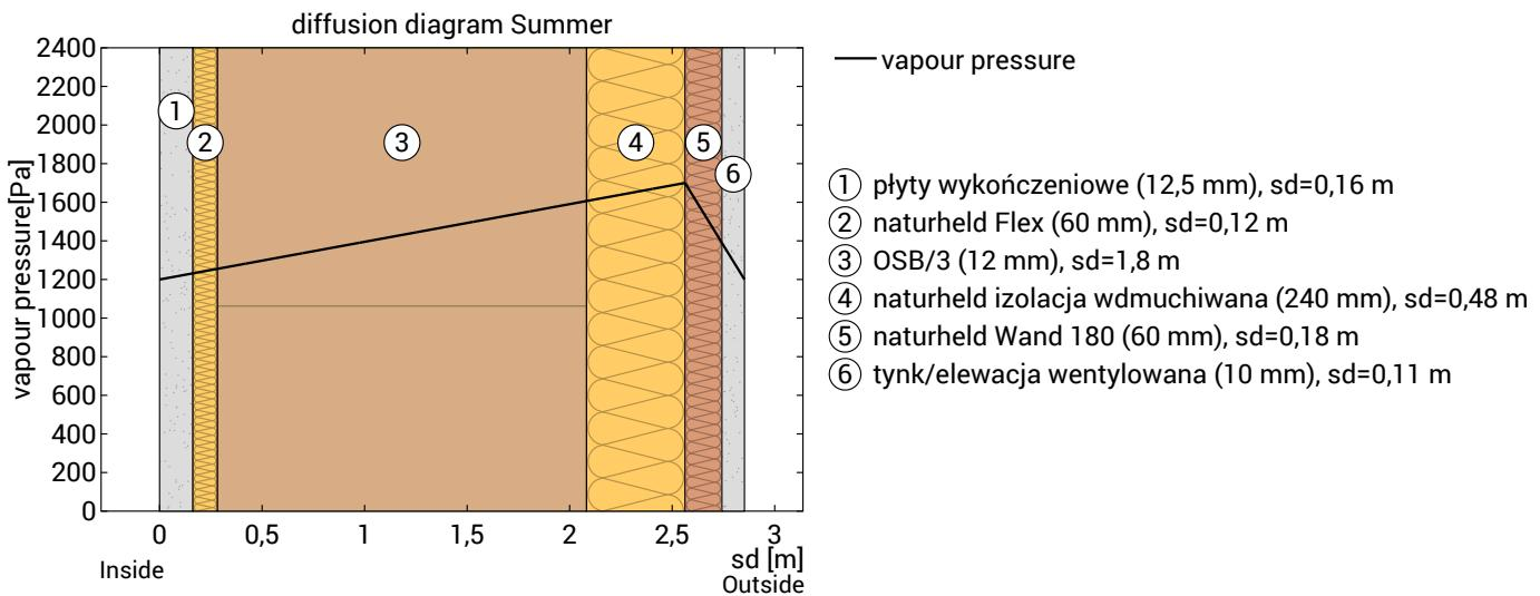
Condensate-free component: The maximum possible evaporation mass for the drying reserve is calculated. Consider the level that has the lowest evaporation potential in the dew period, at sd=2,56 m; x=32,45 cm:
