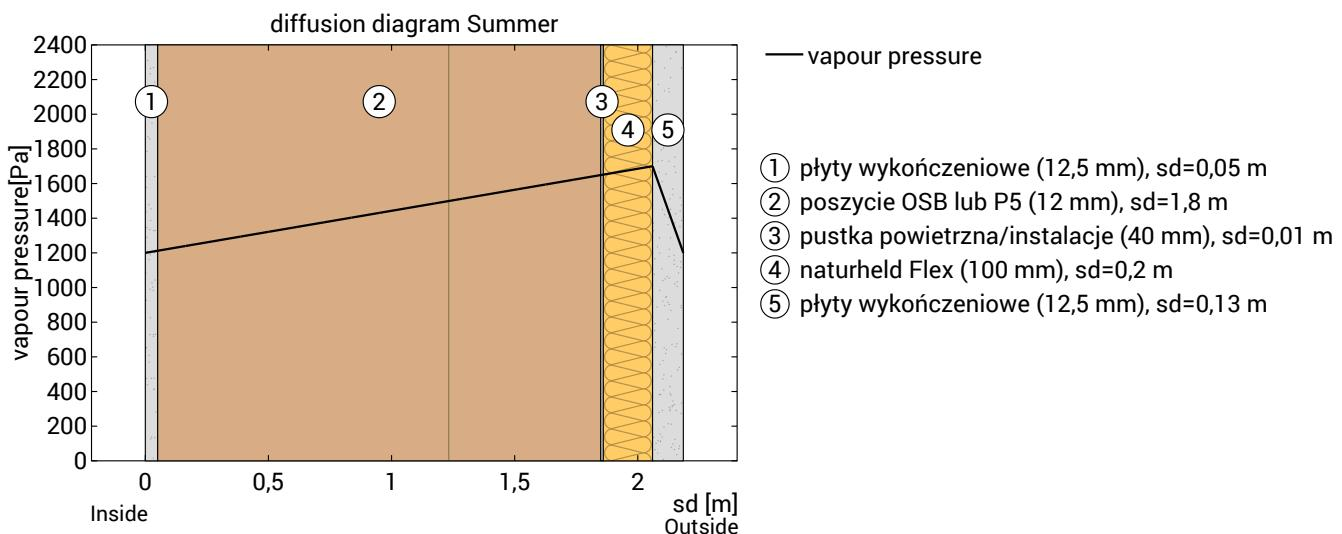
Condensate-free component: The maximum possible evaporation mass for the drying reserve is calculated. Consider the level that has the lowest evaporation potential in the dew period, at  $sd=2,06 \text{ m}$ ;  $x=16,45 \text{ cm}$ :
