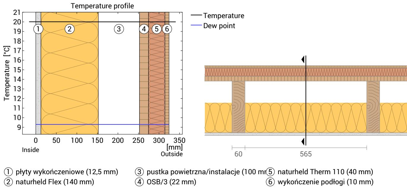
**Left:** Temperature and dew-point temperature at the place marked in the right figure. The dew-point indicates the temperature, at which water vapour condenses. As long as the temperature of the component is everywhere above the dew point, no condensation occurs. If the curves have contact, condensation occurs at the corresponding position.
