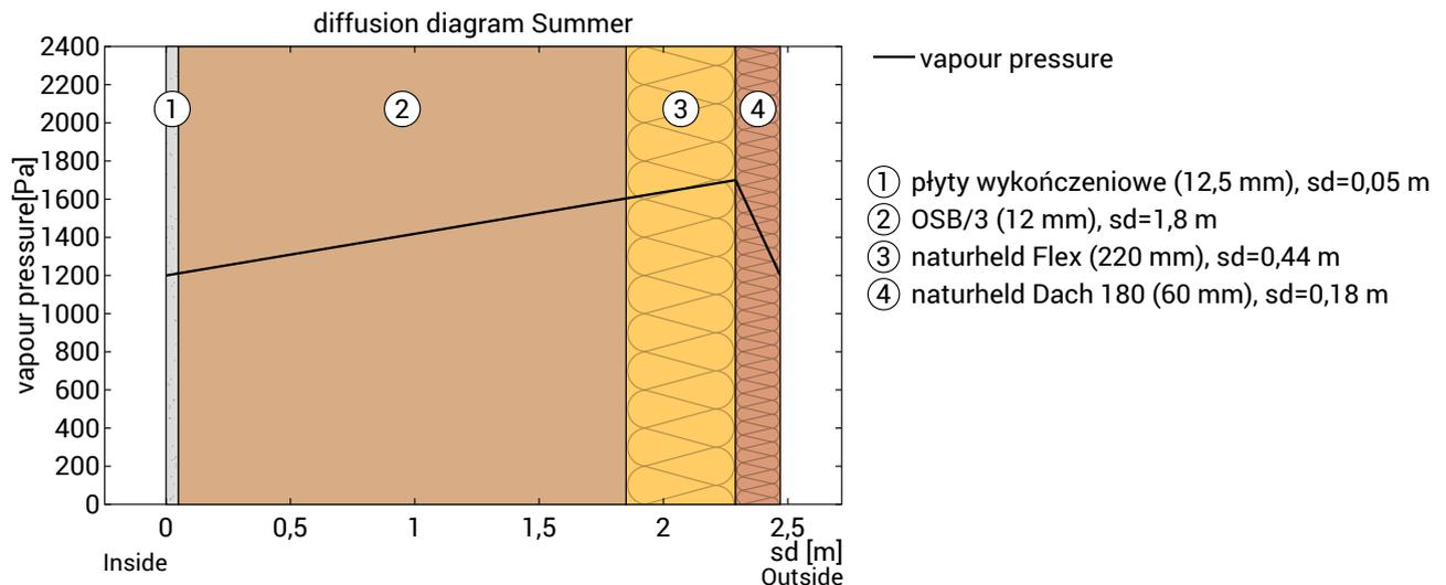
Condensate-free component: The maximum possible evaporation mass for the drying reserve is calculated. Consider the level that has the lowest evaporation potential in the dew period, at sd=2,29 m; x=24,45 cm:
